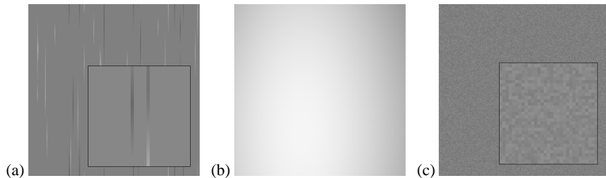
Fig. 8.8. Image degradation: (a) vertical light and dark lines; (b) background level; (c) pixel noise.
