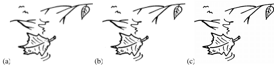
Fig. 9.8. Response of the super-resolution network to a line-drawing: (a) original low resolution image (pixelized); (b) bicubic interpolation (blurred); (c) output of iterative super-resolution network (crisp).
